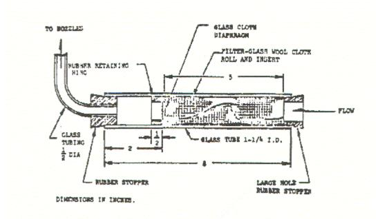
FIGURE 7. Salt solution filter.
