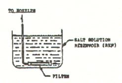
FIGURE 8. Location of salt solution filter in reservoir.
