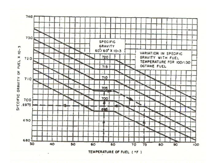
FIGURE 11. Explosive atmosphere fuel weight - temperature characteristics.
