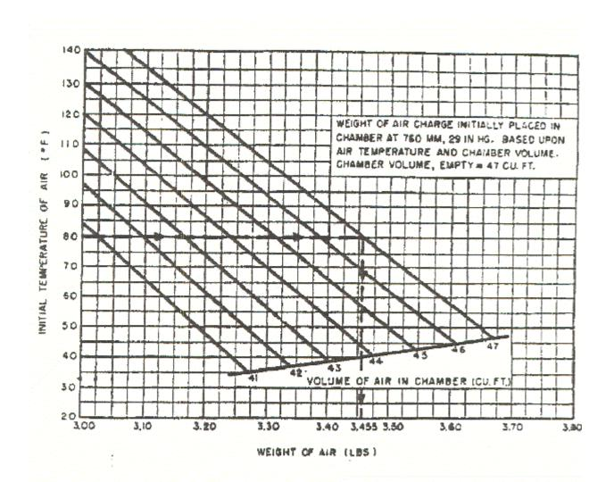
FIGURE 10. Explosive atmosphere air weight - temperature characteristics, chamber volume dependent.
