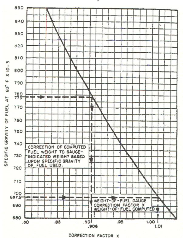
FIGURE 12. Explosive atmosphere fuel weight - temperature characteristic correction factor.
